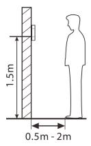
The distance between the device and a user whose height is in a range of 1.55 m to 1.85 m is recommended to be 0.5 m to 2 m. Users may slightly move forward or backward to improve the quality of facial images captured.
