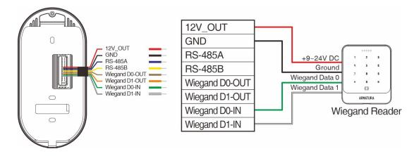
When the device is connected to the controller as a Wiegand reader, the wiring diagram is shown below.
