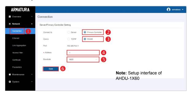
Port: The default system wiring for the primary and secondary controller is RS-485 Port 1.
