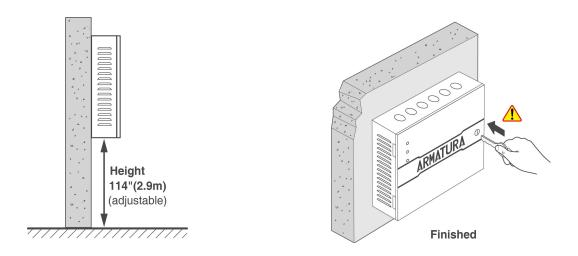
Figure 3-1 Installation the ENC1 enclosure on the wall
