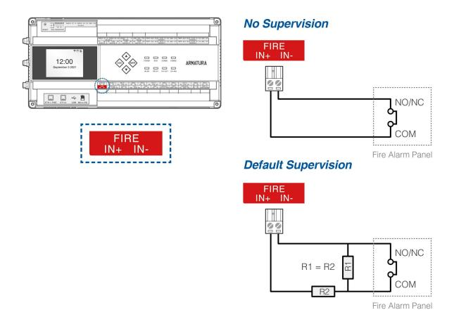
Figure 9-7 Fire Alarm Interface Wiring
