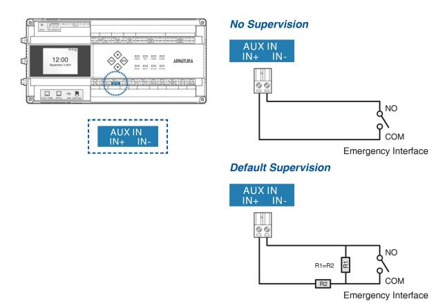
Figure 9-8 Emergency Interface Wiring
