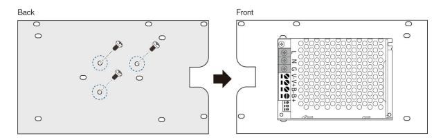
Figure 3-7 Mount the power supply to the mounting plate
