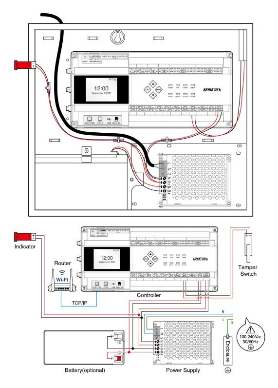
Figure 4-9 ENC1 Enclosure Internal Wiring Diagram
