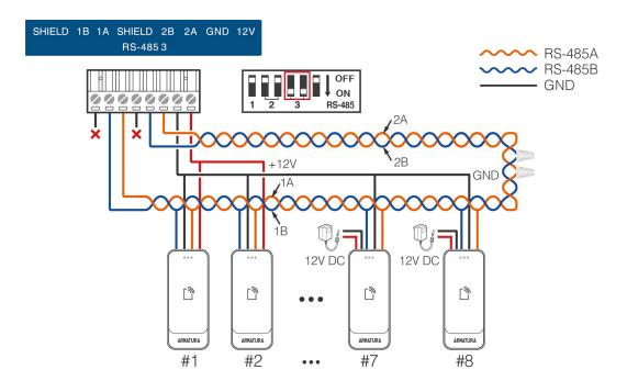
Figure 4-20 RS-485 redundancy backup connection of controller and RS-485 readers
