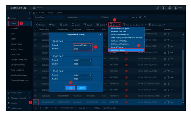
Device has three physical interface, RS-485 Port 1/Port 2/Port 3.
