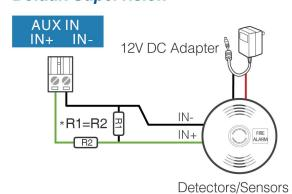
Figure 4-13 Auxiliary Input Wiring
