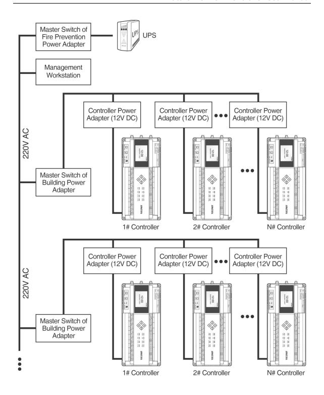
Figure 3-13 Access Controller System Power Supply
