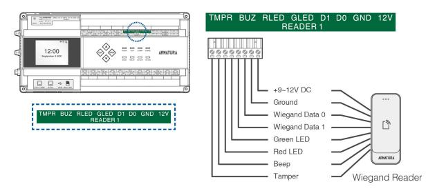
Figure 4-15 Wiegand Reader Wiring
