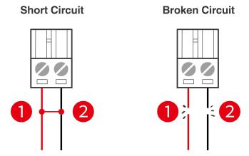
Figure 4-24 Line monitoring diagram
