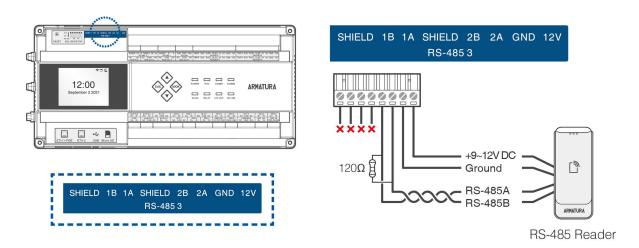
Figure 4-18 RS-485 Reader Wiring
