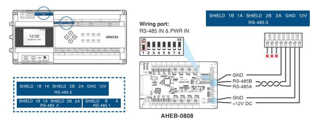
Figure 4-21 I/O Board Wiring
