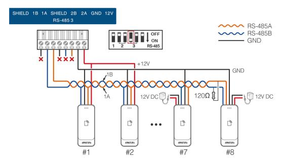
Figure 4-19 Hand-to-hand connection of controller and RS-485 readers
