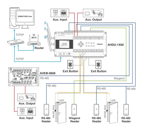
Figure 3-11 Schematic Diagram of AHDU-1X60 System Installation
