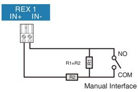
Figure 9-9 Manual Interface Wiring
