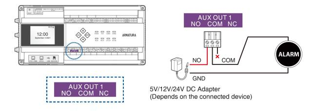
Figure 9-10 Alarm Output Interface Wiring
