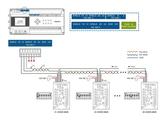
Figure 9-6 Hand-to-hand connection of multiple I/O board
