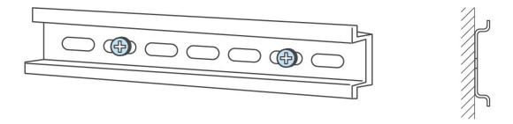
Figure 3-3 Mount the DIN rail
