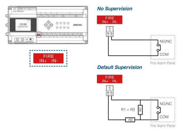
Figure 4-17 Fire Alarm Monitoring Wiring
