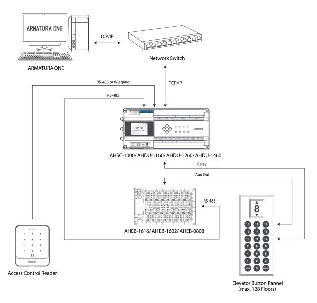
Figure 9-1 Elevator Control System Wiring Diagram
