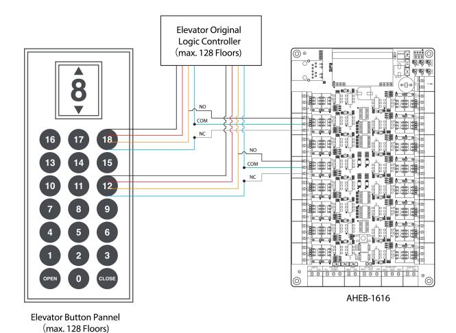
Figure 9-3 AHEB-1616 Wiring Diagram with Elevator Panel
