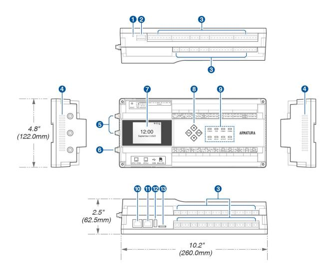
Figure 2-2 AHDU-1X60 Secondary Controller Appearance
