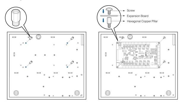
Figure 3-2 Schematic diagram of screw installation
