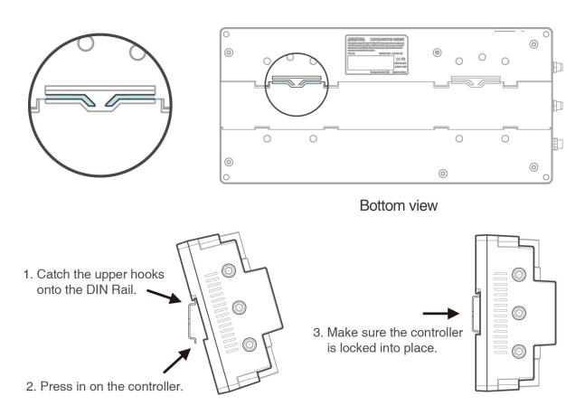
Figure 3-4 Mount the controller to the DIN rail adapter
