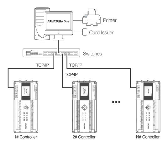
Figure 5-1 TCP/IP Communication System Networking
