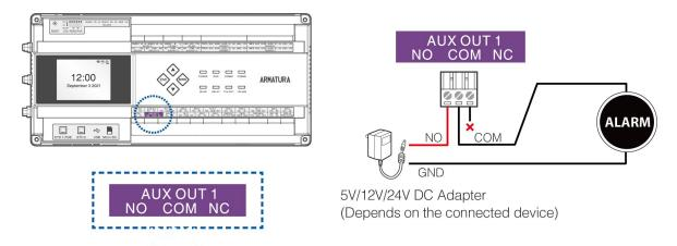
Figure 4-12 Auxiliary Output Wiring
