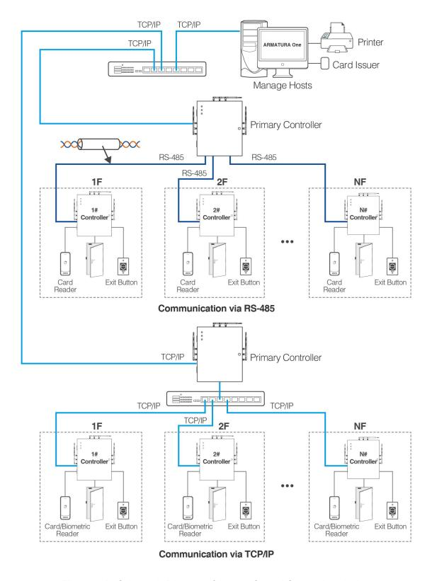
Figure 3-10 Schematic Diagram of Access Control System Installation
