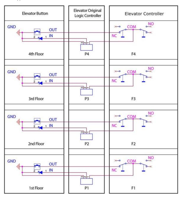
3. Wiring method when there are multiple identical buttons on the same floor.
