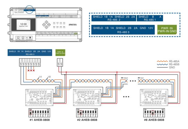
Figure 4-22 I/O Board Wiring
