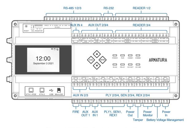
Figure 4-1 AHDU-1X60 Terminal connection diagram
