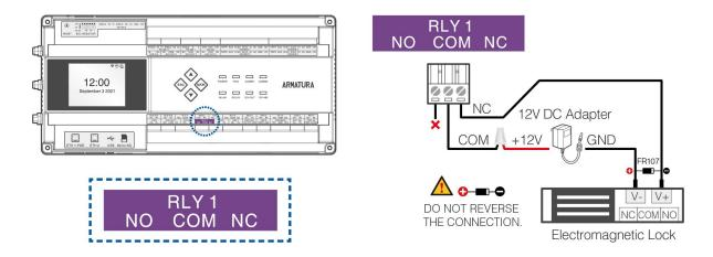
Figure 4-16 Wiring diagram of lock connection
