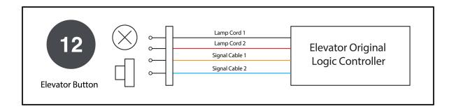
Figure 9-4 Elevator button wiring schematic
