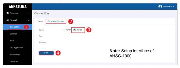
**Port:** This is the RS-485 port used for connecting the secondary controller. The specific port to be used depends on the setting in Armatura RS-485 Port Settings.
