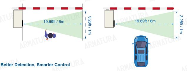
Advanced Radar Technology: Ensures high detection accuracy with minimal false alarms.
